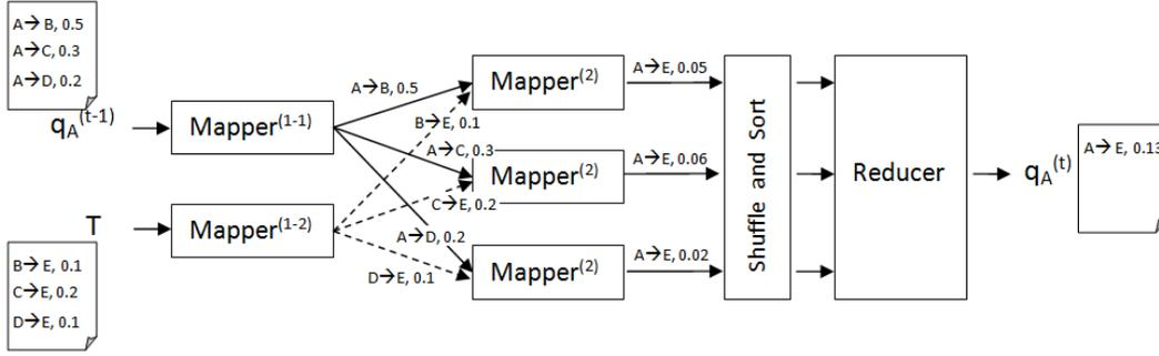
Figure 2: One iteration of random walk in the MapReduce framework. Pair of edges to be connected are distributed to the same mapper which joins them based on the common vertex to emit a new edge. The reducer aggregates intermediate instances of “A →E” to generate the complete edge.
