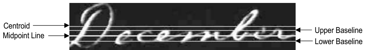
Figure 3: Diagram demonstrating the possible cross-section rows.
