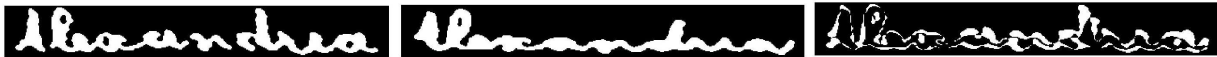
Figure 9: Two examples of “Alexandria,” after preprocessing. On the right is the corresponding XOR image. The white pixels in the XOR image represent mismatched pixels.
